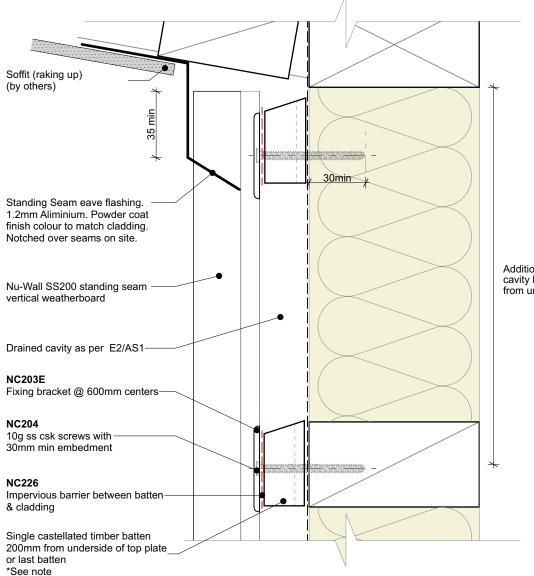
Additional nog and castellated cavity batten to be 200mm max from underside of top plate
