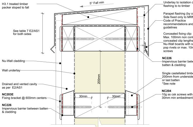
Underlay to isolation of metal flashing to to timber
