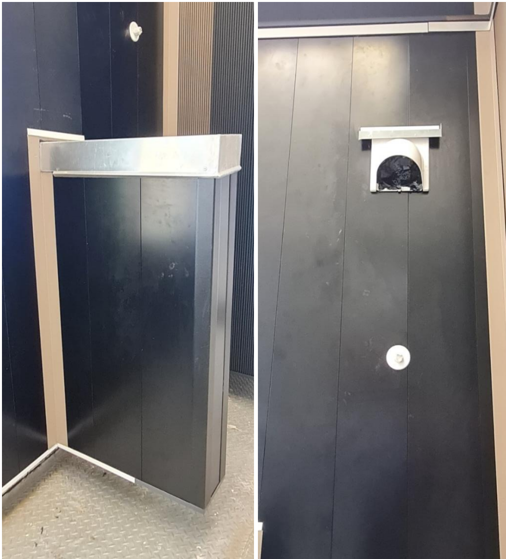
Figure 28: Balustrade/parapet, large pipe cowl, and small pipe flange
